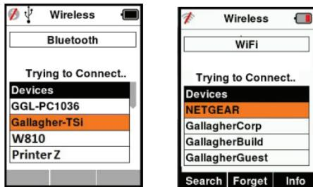
**Note:** The HR4 can be configured to send and/or receive data from other devices via Bluetooth and WiFi.
